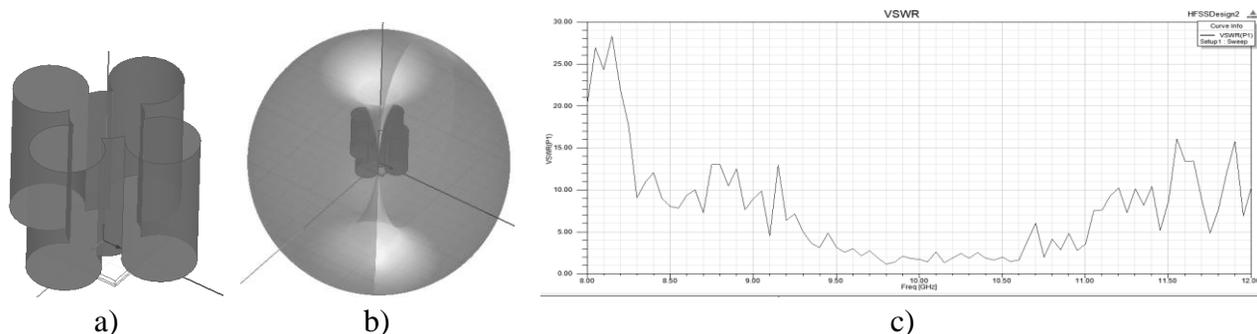
Fig. 3. The second version of quasifractal DRA: a) – power circuit; b) – BP; c) – frequency dependence of a SWR
