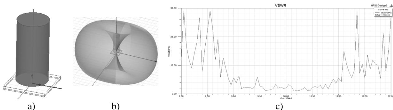
Fig. 1. Basic element of the DRA on the basis of a cylinder: a) – power circuit; b) – BP; c) – frequency dependence of a SWR
