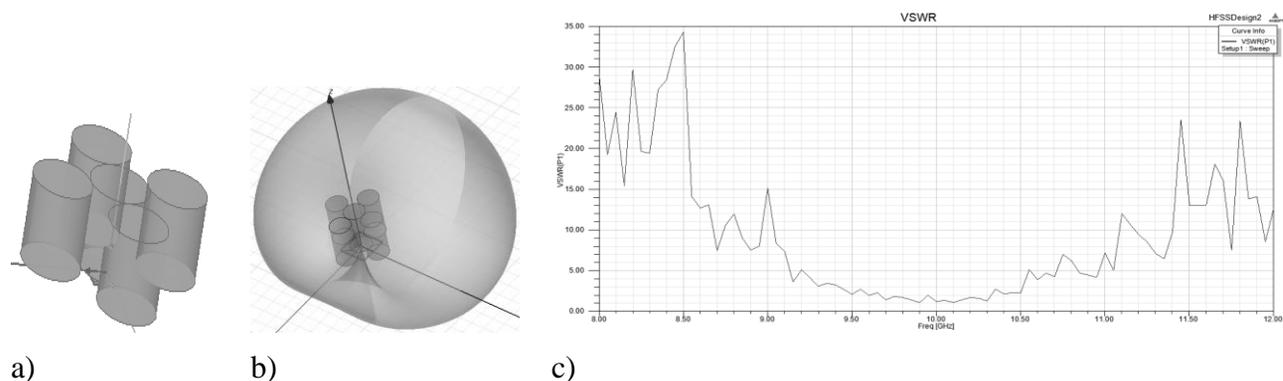
Fig. 2. The first version of quasifractal DRA: a) – power circuit; b) – BP; c) – frequency dependence of a SWR
