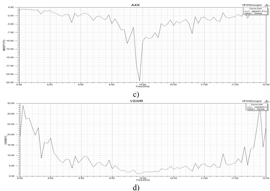
**Fig. 4. Third version of quasifractal DRA: a) – power circuit; b) – BP; c) – AFC; d) – SWR**
