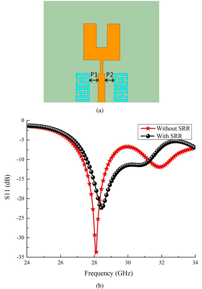
Fig. 5. SRR loaded antenna configuration (a) Layout (b) Reflection coefficient ( $P_1 = P_2 = 1mm$ ).
