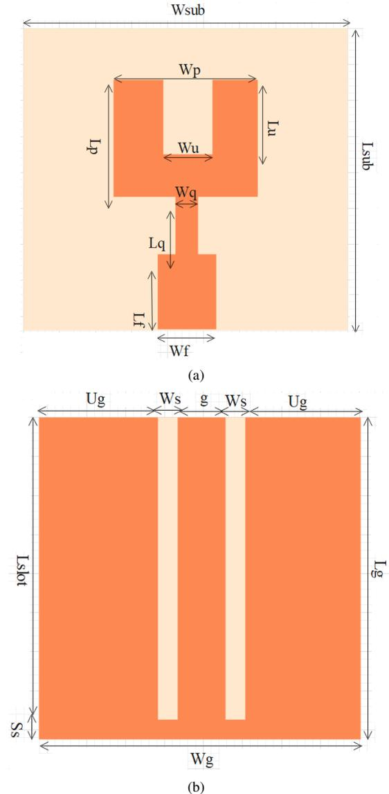
Fig. 1. Layout of the antenna configurations (a) Top view (b) Bottom view.
