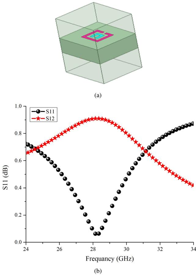
Fig. 4. Characterization of SRR (a) Simulation setup in high-frequency-structural-simulator (b) Reflection coefficients, S11 and S12.
