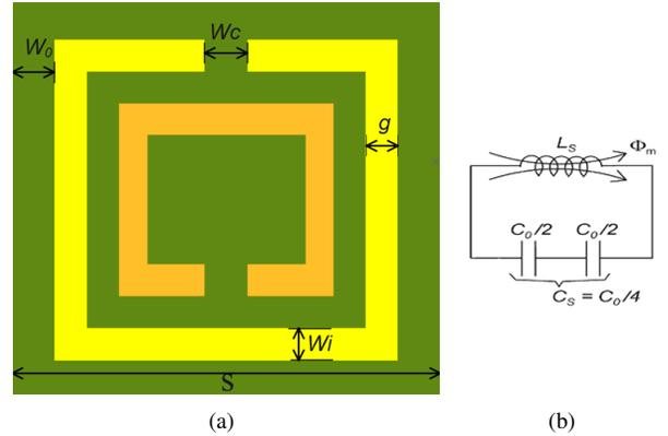
Fig. 3. Split-ring-resonator and its equivalent circuit (a) Layout (b) Equivalent circuit.
