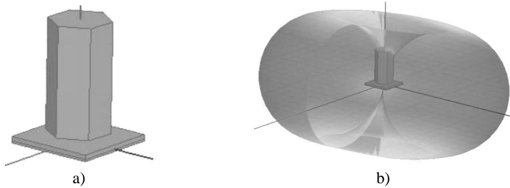
Fig. 1. Basic element DRA based on on a hexagon: a) – power scheme; b) – BP
