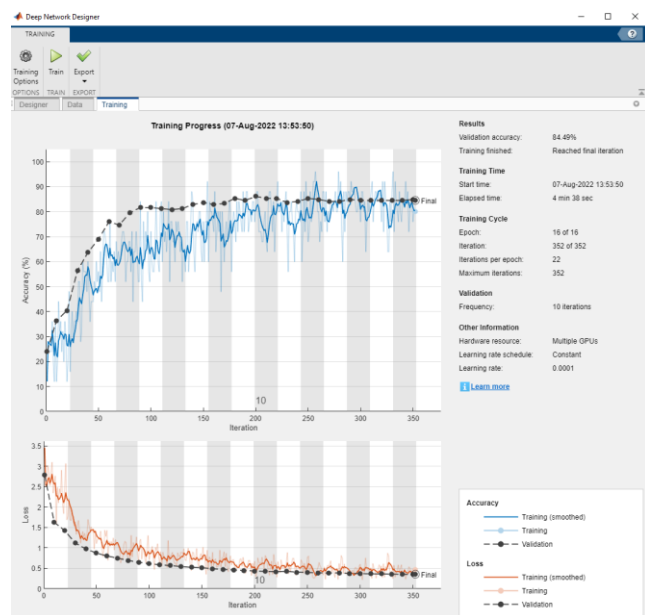
Fig. 11. Assessment of classification accuracy of validation (test) sampling – 84%, Epoch 18, Iteration 352
